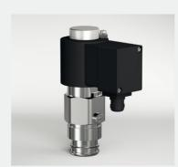
The pilot operated high-pressure solenoid valve made of stainless steel for screw fitting can safely control pressures up to 300 bar. Special versions are designed for pressures up to 900.
